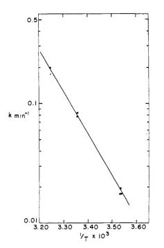
Figure 3. Arrhenius plot of the rate of decarboxylation of N-carboxy-2-imidazolidone at pD 7.4.
