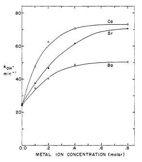
Figure 4. Effect of metal ion concentration on the rate of saponification of N-p-nitrophenoxycarbonyl-2-imidazolidone at  $25^{\circ}$ . Rates expressed as second-order rate constants obtained by dividing the observed pseudo-first-order rate constant by the added hydroxide ion concentration. Hydroxide ion concentrations employed were 0.0106, 0.0109, and 0.00778 *M* in the strontium, barium, and calcium reactions. Each point is the average of two rate measurements which deviated by less than 10%.
