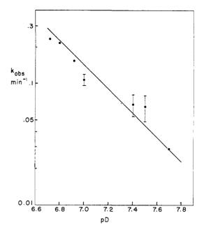
Figure 2. Rate of decarboxylation of N-carboxy-2-imidazolidone as a function of pD at  $25^{\circ}$ . Vertical bars represent the average deviation in cases where more than one determination was made. The slope of the line is 1.0.
